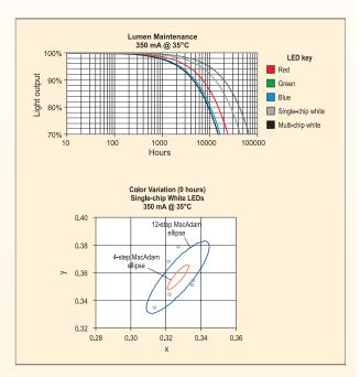
Top: Actual (to 10,000 hours) and estimated (beyond 10,000 hours) light output change over time. The trend lines indicate approximately when each LED will reach 70% of initial light output. Bottom: Initial color variation between each white LED in one single-chip LED array.
