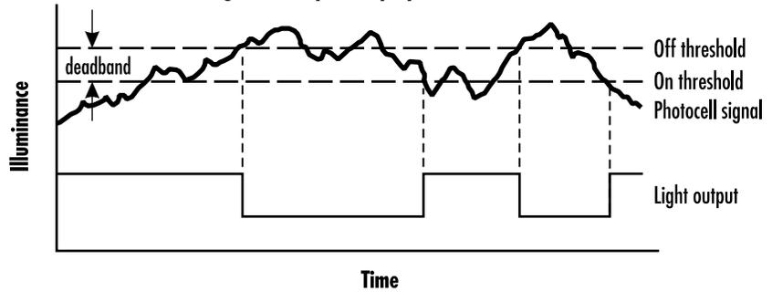
**Figure 3c. Deadband for closed-loop systems**
