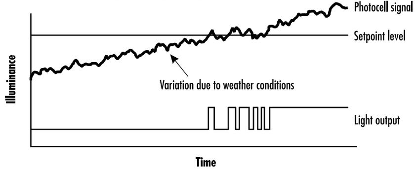
**Figure 3b. Open-loop systems with deadband**
