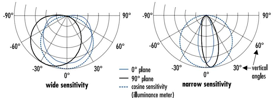
These curves depict a photosensor with a wide sensitivity and a photosensor with a narrow sensitivity. The cosine sensitivity is shown to compare the sensitivity curve to that of an illuminance meter.
