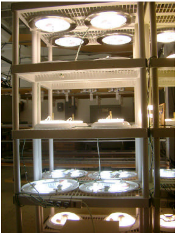
Figure 8. Voltage pilot test apparatus
