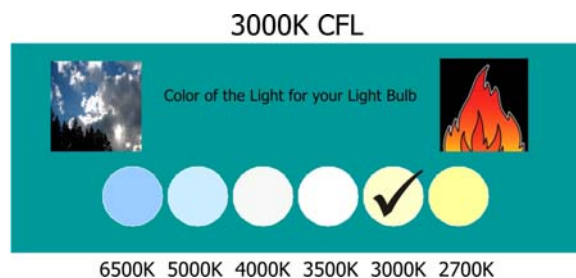
Figure 7. Proposed package illustration for a fluorescent lamp with a correlated color temperature (CCT) of 3000 K, indicated by the check mark. The colored discs in the illustration correspond to the six CCTs designated for linear fluorescent lamps by ANSI. The two icons, daylight and fire, are intended to represent the two extremes in chromaticity space for “white” light sources.
