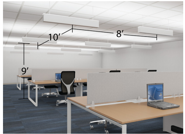
Figure 2. Typical office space assumed for the calculations shown in the lookup table.
