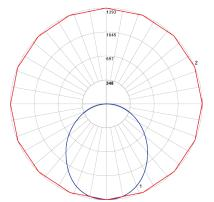
Figure 3. Photometric distribution of the direct luminaire employed for the calculations in the lookup table.
