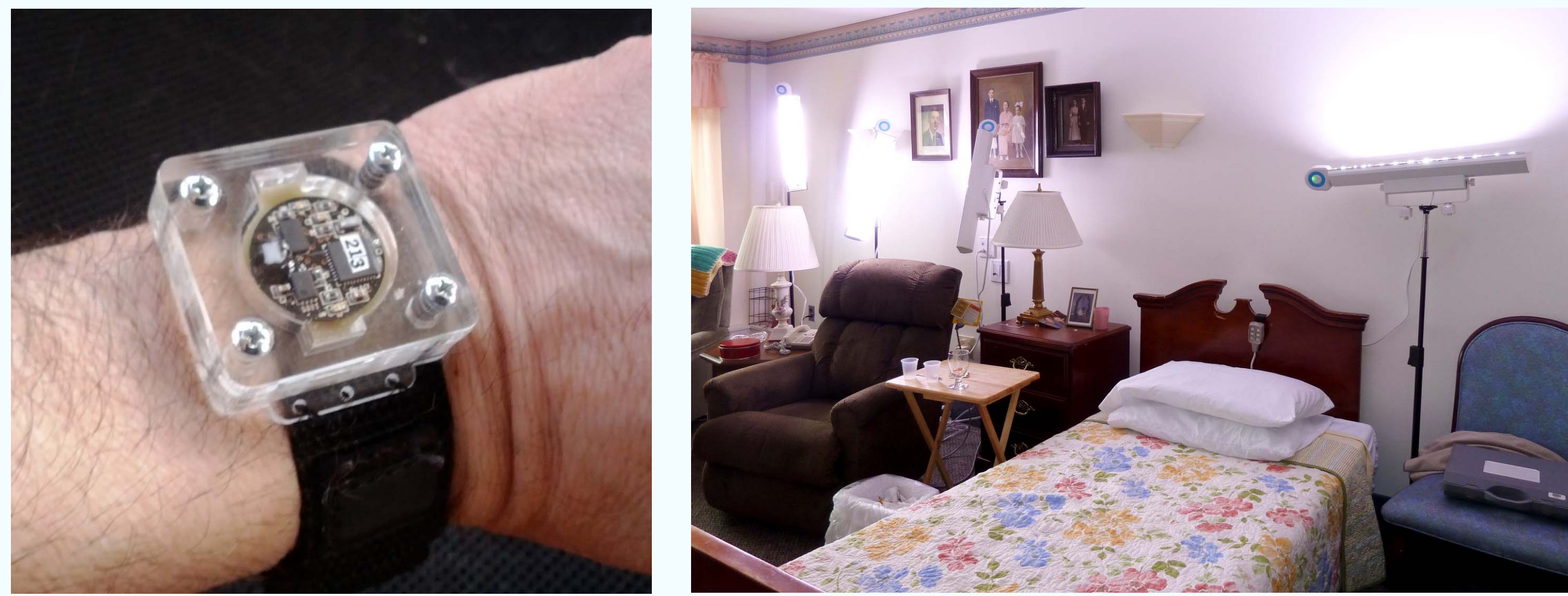
Figure 1. The Daysimeter (left), worn on the wrist, was used to record calibrated light and activity levels. The tailored lighting intervention used that was installed in a patient's room (right) used two GE 45851 F55BX/AR/FS fluorescent lamps inserted in a luminaire head (Elco Lighting, ETC 454, Line Voltage T5 Fluorescent Wall Washer).
