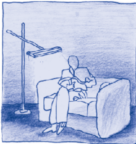
Place a task light over the reader's shoulder, close to where he/she reads.
