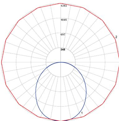
Figure 3. Photometric distribution of the direct luminaire employed for the calculations in the lookup table.
