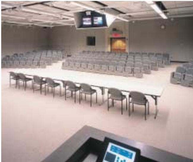
Direct lighting, without wallwashing (looking toward rear)
