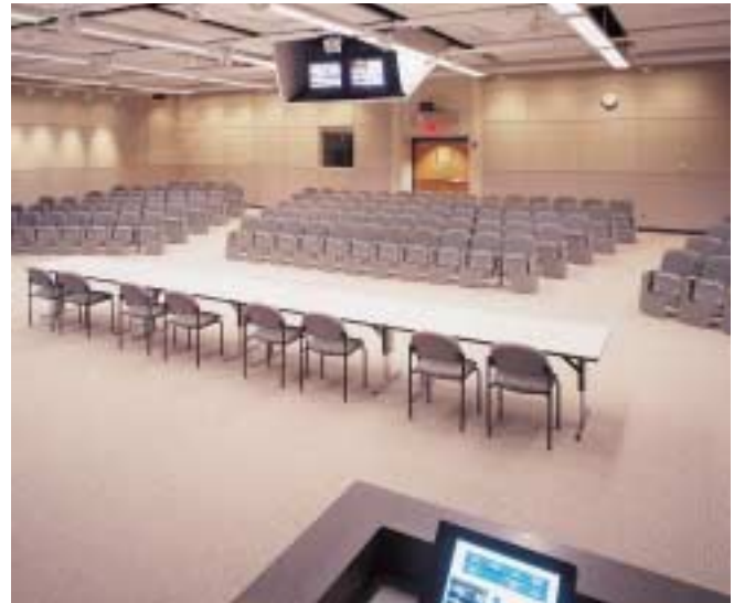
Direct lighting, with wallwashing (looking toward rear)
