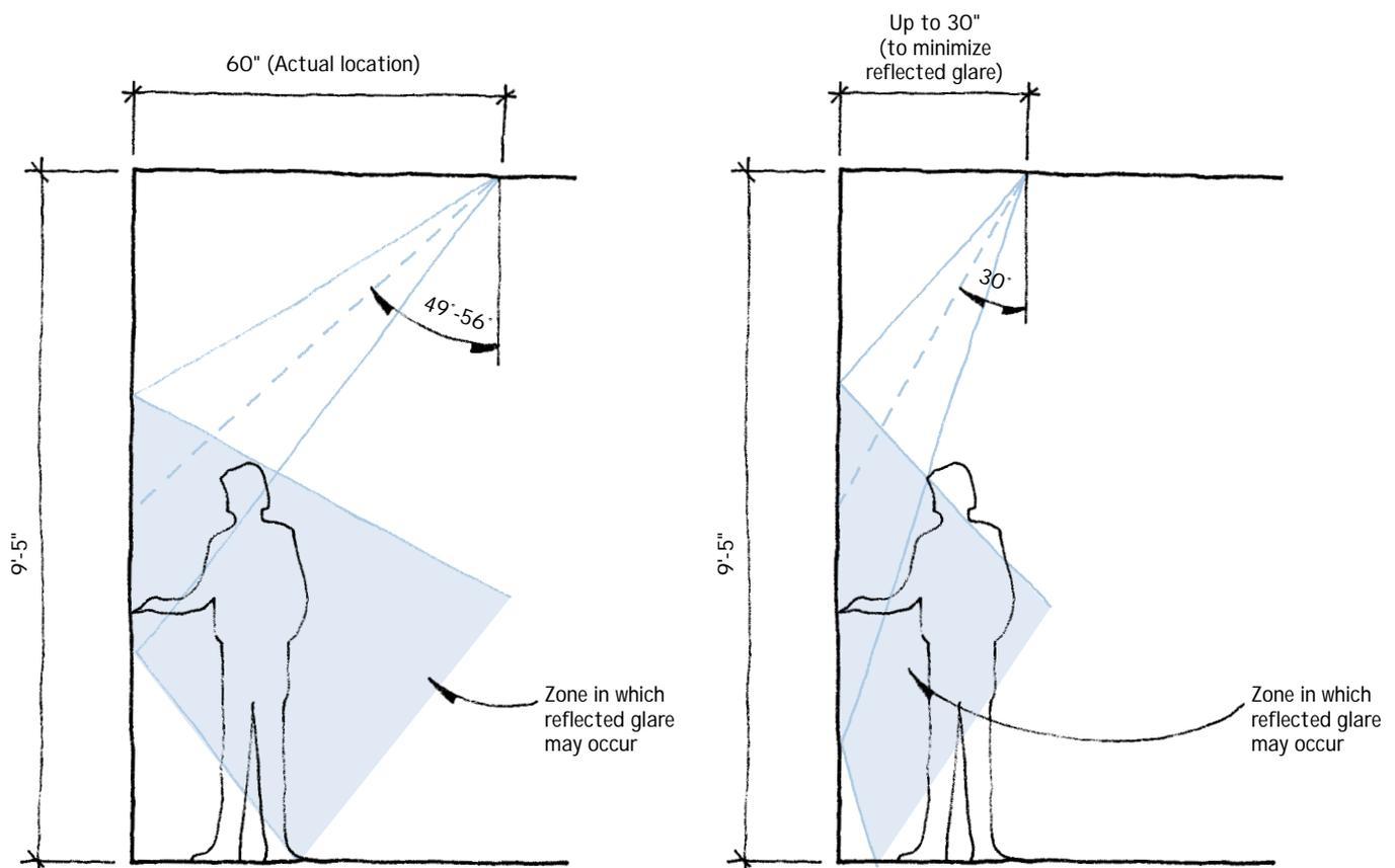
Reflected glare on a glossy whiteboard can occur when a luminaire is mounted at a distance greater than 30 inches from the board.
