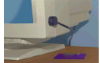
Manual dimmer mounted on computer monitor
