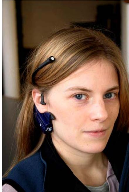
Do not let the Daysimeter point up (as shown) or down.
