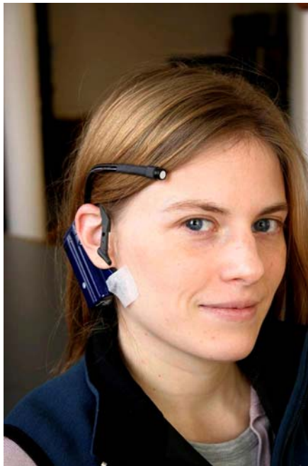
Adhesive tape may be used to hold the Daysimeter in place.
