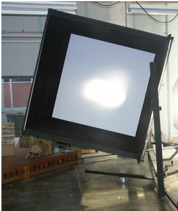
Fig. 3: Configuration to avoid interreflections: one white panel and four black panels
