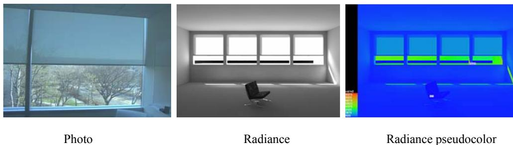
Fig. 7: Comparison of the actual and rendering images of roller shade
