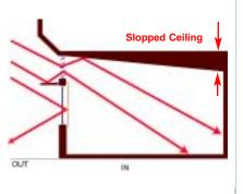
has a 38 foot outside wall, a 38' x 2'-8" aperture will provide enough glass. However, if the 26'-4" dimension is on the outside wall, and the glass is still 2'-8" tall, you will only be able to achieve a 7% glass-to-floor area ratio - not enough to effectively daylight the space.
