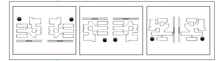
As you can see, the classroom wings, under any scenario, run east-west in length with roof monitors facing south or north. The rest of the building core was developed so that square roof monitors could be rotated within the same space, always facing south.
