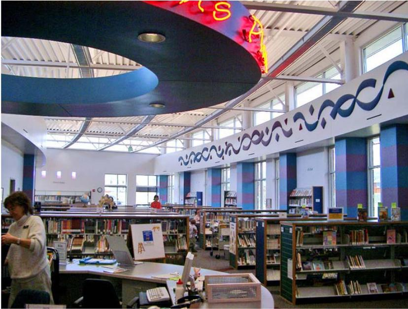
*On the northwest side of the Children's Place there is insufficient shading for some times of day. One clerestory window allows a shaft of sun to penetrate deep into the space where librarians are stationed.*
