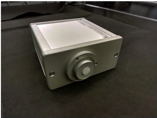
Figure 5. Commercial spectroradiometer capable of measuring irradiance in the 200 nm to 430 nm range
