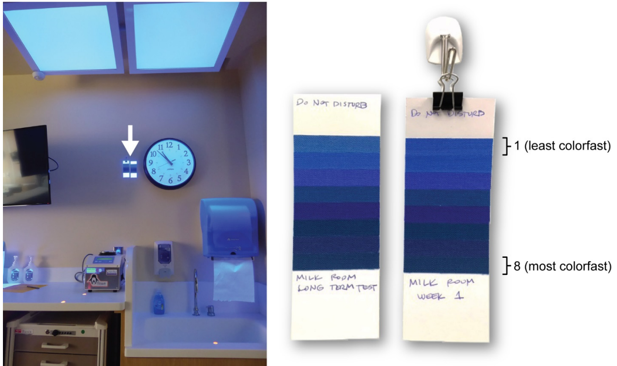
Figure 10. Blue wool test of colorfastness at a UV-A installation
