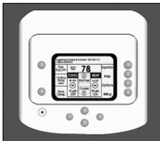
Figure 1 Programmable control pad for DDC manual control
