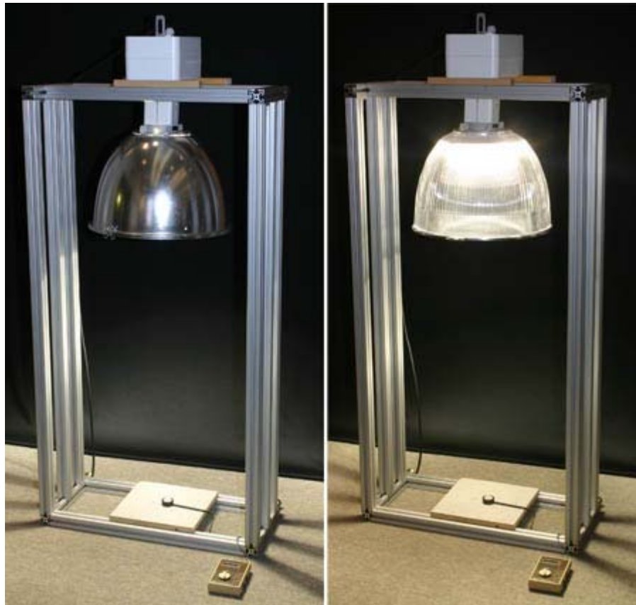
Figure App-1. Luminaire and reflectors used for thermal testing - Specular aluminum reflector (left) and acrylic prismatic refractor (right)
