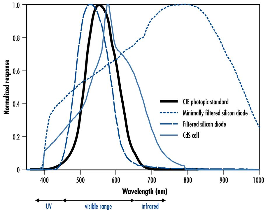
The graph shows how the response of different detection types compare to the photopic luminous efficiency function, which defines the measurement of light. The detector types are shown in the graph legend.
