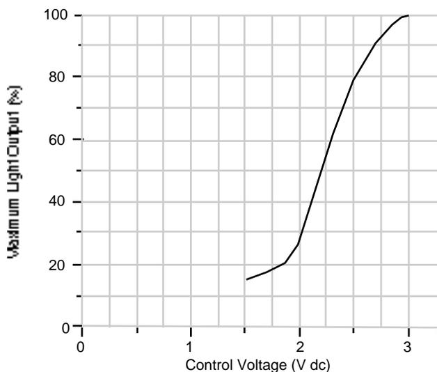
Response characteristics of the ETTA EC2S-120A8D dimming electronic ballast, as tested by NLPIP.
