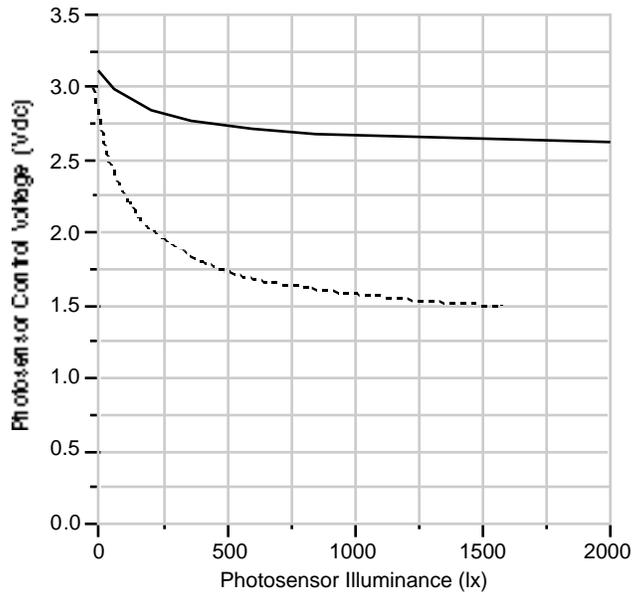
Response functions at the maximum (—) and minimum (---) sensitivity settings of the ETТА photosensor, as tested by NLPPI.
