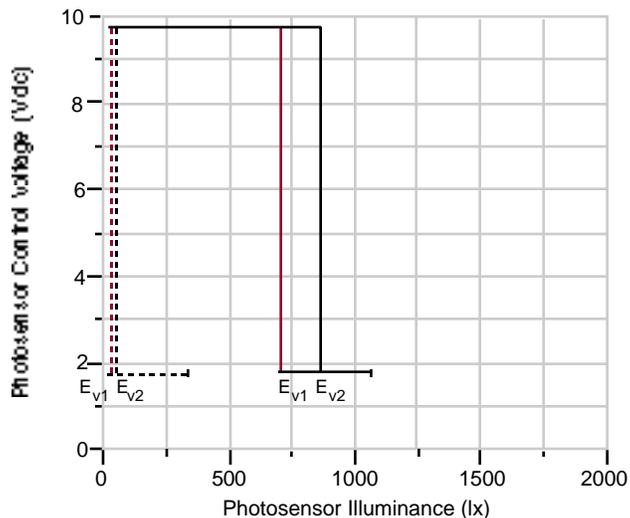
Response functions at the maximum (broken lines) and minimum (solid lines) sensitivity settings of the Watt Stopper photosensor, as tested by NLPIP. NLPIP measured and recorded data at individual points until the photosensor began to respond. NLPIP then recorded the voltage at which the photosensor stabilized.
