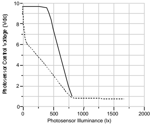
Response functions at maximum (---) and minimum (—) sensitivity settings of the UNENCO photosensor, as tested by NLPiP.
