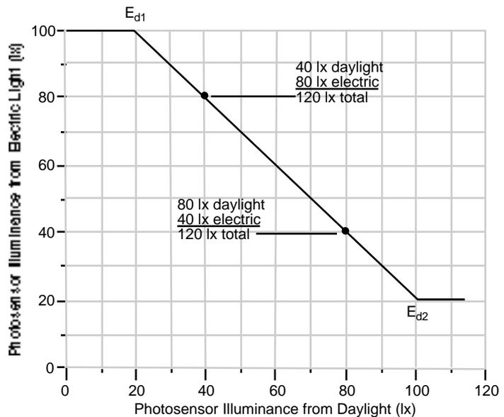
Example of a response function for a threshold-response photosensor-controlled lighting system (illuminance from the electric lighting system alone versus photosensor illuminance provided by daylight alone) for a daylighting application.
