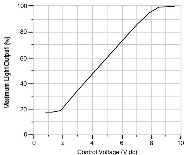
Response characteristics of the Advance Mark VII dimming electronic ballast, as tested by NLPIP.
