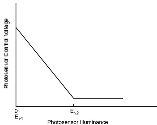
The figures show that the ballasts both have nearly linear responses between two voltages. NLPIP calls the range between these two voltages the *control voltage response range*. The table below gives the control voltage response ranges for several dimming electronic ballasts for T8 fluorescent lamps, as measured by NLPIP.
