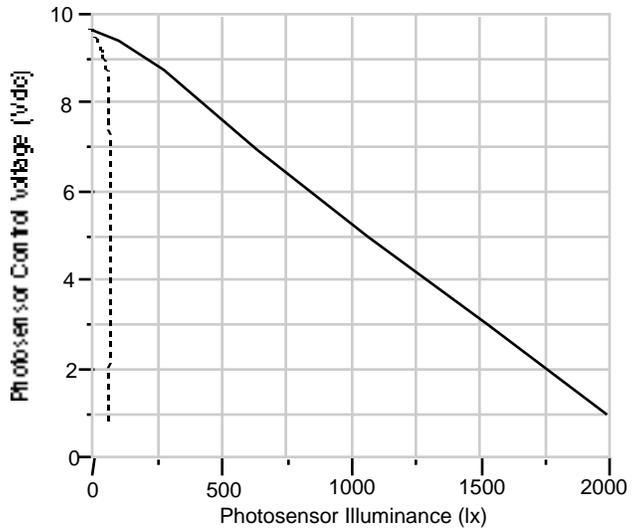
Response functions at the maximum (---) and minimum (-) sensitivity settings of the Sensor Switch photosensor, as tested by NLPIP.
