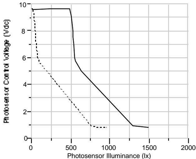
Response functions at the maximum (—) and minimum (---) sensitivity settings of the Honeywell photosensor, as tested by NLPPI.
