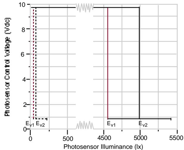
Response functions at the maximum (broken lines) and minimum (solid lines) sensitivity settings of the PLC MULTIPPOINT photosensor, as tested by NLPIP. NLPIP measured and recorded data at individual points until the photosensor began to respond. NLPIP then recorded the voltage at which the photosensor stabilized.
