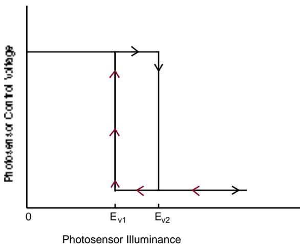
**Figure 3. Response Function of a Hypothetical Continuous-Response Photosensor**
