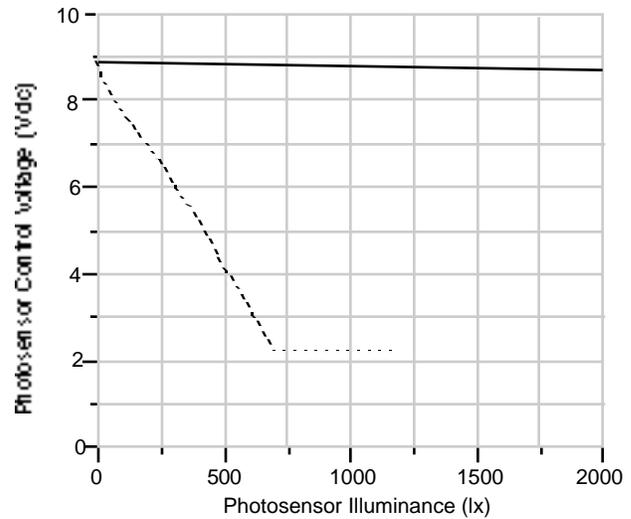
Response functions at maximum (---) and minimum (—) sensitivity settings of the Lutron photosensor, as tested by NLPiP.
