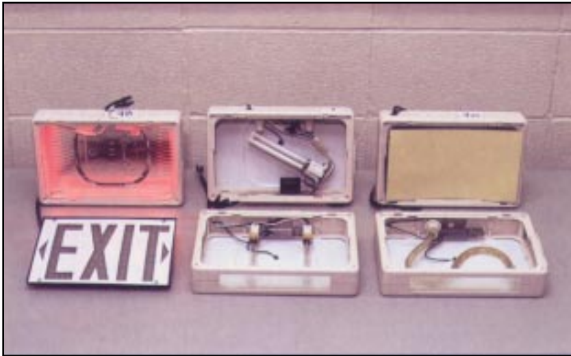
Interior of exit signs, showing retrofit kits. Clockwise, from upper left: side-mounted LEDs, compact fluorescent lamp, electroluminescent panel, incandescent light tube, incandescent lamps, LED replacement faceplate.
