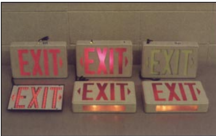
Retrofit kits installed in host sign. Clockwise, from upper left: side-mounted LEDs, compact fluorescent lamp, electroluminescent panel, incandescent light tube, incandescent lamps, LED replacement faceplate.
