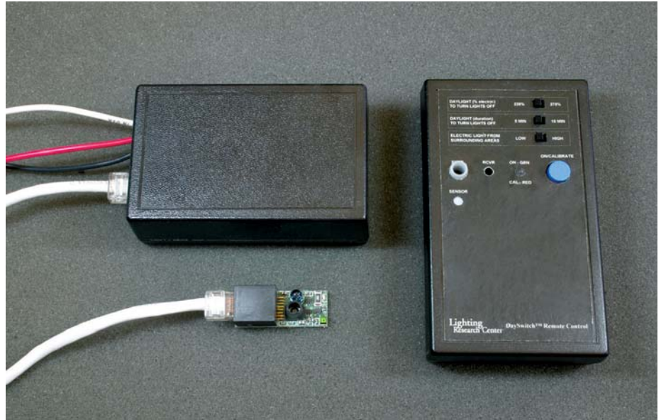
The three elements of the DaySwitch (clockwise, from upper left): control module, remote commissioning device, and sensor module
