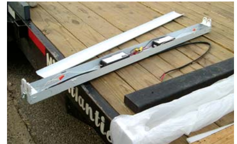
The fluorescent luminaire is ready for field installation. The white plastic diffuser is in the foreground.
