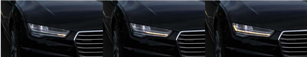
This front turn signal, when activated, gradually illuminates from the vehicle's center outward, providing additional cues about the intended turn direction.
