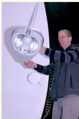
An LRC researcher mounts a cobra head fixture containing a mogul base LED lamp for testing inside an integrating sphere.
