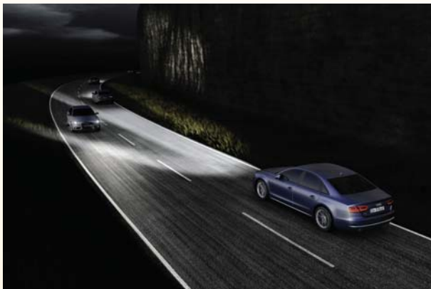
Artist's rendering. Note how the bright headlamp beam avoids the oncoming car. (Image courtesy of Audi AG.)
