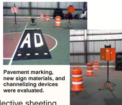
Pavement marking, new sign materials, and channelizing devices were evaluated.
