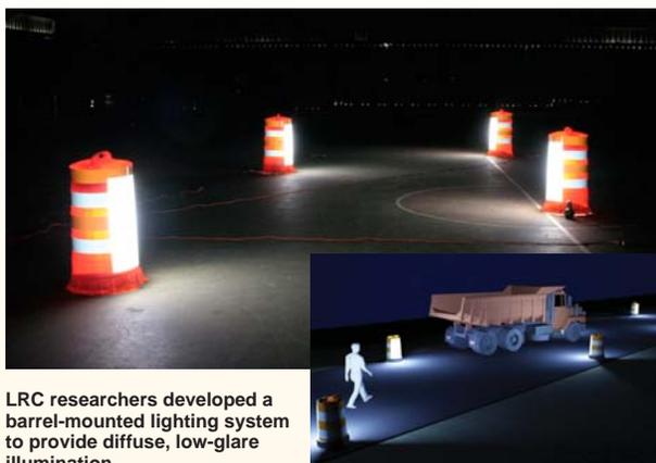
LRC researchers developed a barrel-mounted lighting system to provide diffuse, low-glare illumination.
