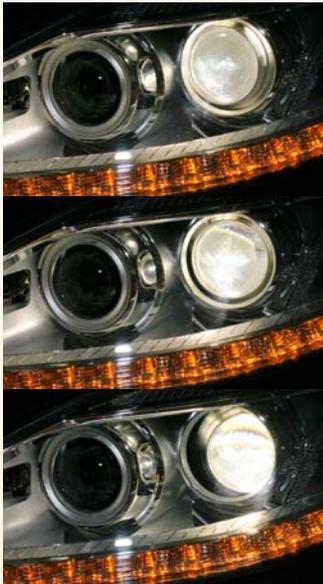
Swiveling headlamps like these can aim their beam  $\pm 15^\circ$  to left or right of the center position.
