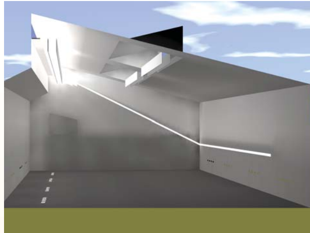
Lighting simulation using AGI32 illustrates that daylight penetration into workbay spaces is better controlled when interior baffles and light shelves are specified.
