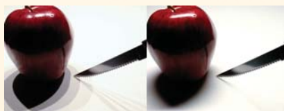
Discrete shadows produced by LED luminaires vs. soft shadows produced by fluorescent luminaires.
