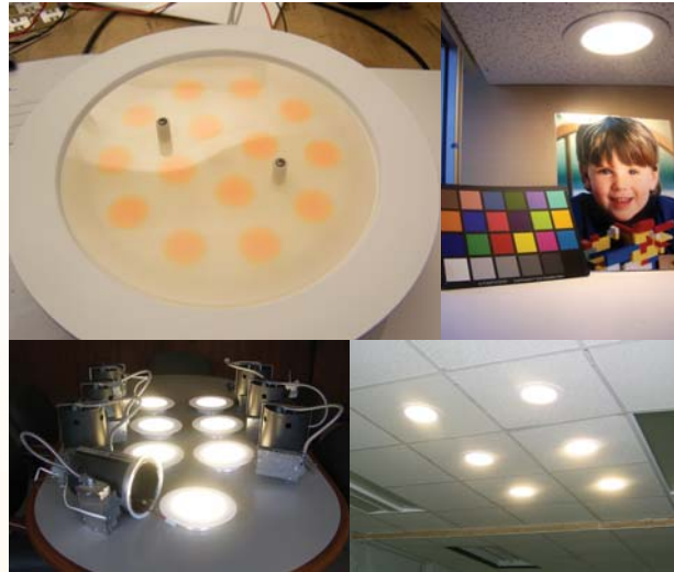
Top left: prototype SPE LED downlight; top right: prototype color rendering; bottom left: seven prototypes built for the project; bottom right: six prototypes installed at the LRC.
