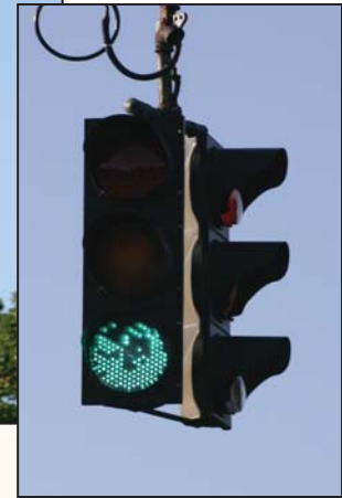
Examples of failed LED traffic signals.
