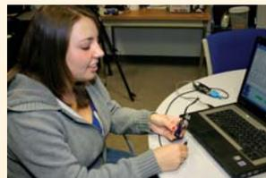
A student researcher gathers data from a Daysimeter, a light-measuring device developed at the LRC.
