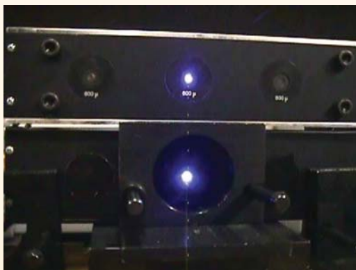
View of apparatus showing LED (top) and filtered incandescent (bottom) signal lights
