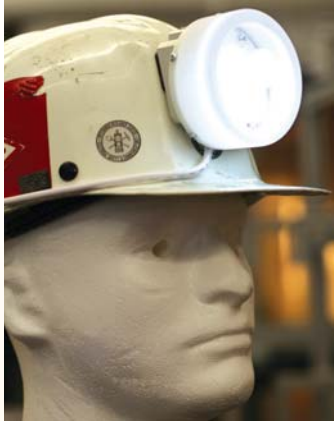
LED helmet lighting prototype developed by the LRC project team.
