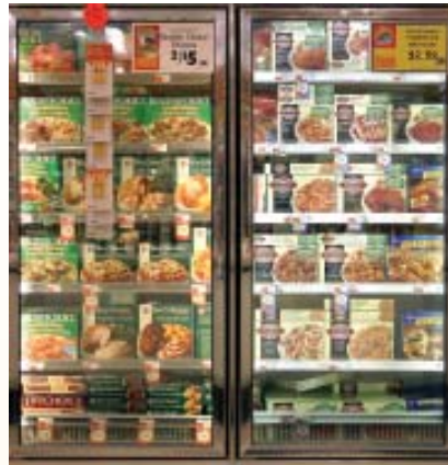
The photo shows the test fluorescent-lit freezer on the left, and the LED-lit freezer on the right. The LED-lit freezer showed better light uniformity across the width of the shelves, leading to better ratings from shoppers.
