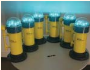
Prototype airport fixtures developed by the LRC are used in flight tests in Alaska and North Dakota to validate laboratory results. Placed at the corners of an airport runway, these fixtures help to confirm the optimum spectrum, intensity, flash rate, and distribution for airport lighting.
