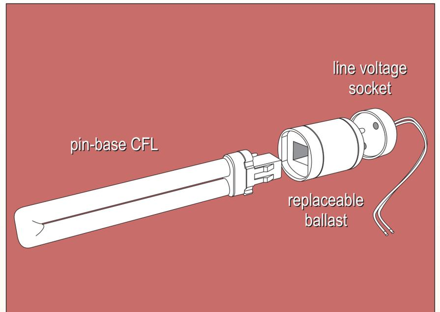
Replaceable electronic ballasts for ENERGY STAR residential luminaires are becoming more popular. Currently, no design standard exists for line-voltage sockets (i.e., what the replaceable ballast plugs into). The lack of a standard socket means that when the replaceable ballast dies, consumers must find the correct replacement that fits their luminaire's particular socket. Difficulties with buying replacement parts can limit product acceptance.
