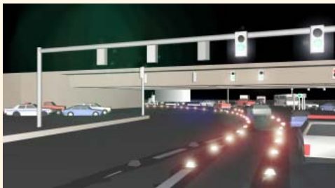
LRC rendering of a proposed SPUI viewed from a vehicle at an intersection using LED markers.
