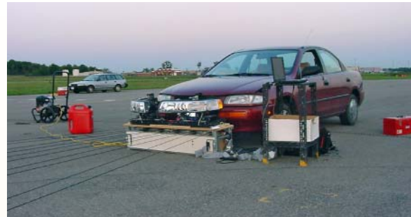
Test vehicle positioned behind adjustable headlamps on a test stand.
