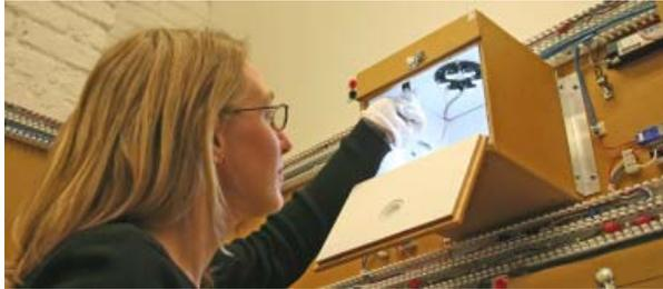
For any fixture and lamp, life is an issue. How long will a lamp continue to shine? At what point is its quality and quantity of light output no longer acceptable? Although high-power LEDs generally perform better than previous types, each type and color of LED may perform differently. The LRC is learning more about how LED characteristics change over time.
