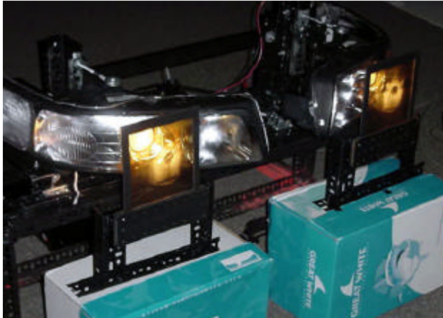
Figure 3. Headlamp rack assembly with filters.
