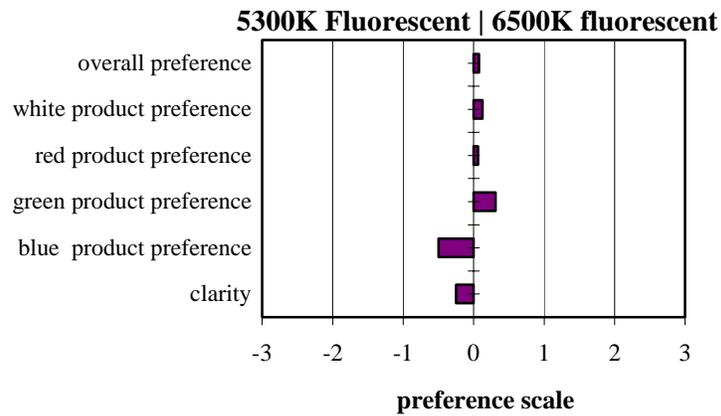
**Figure 9:** Color temperature test results
