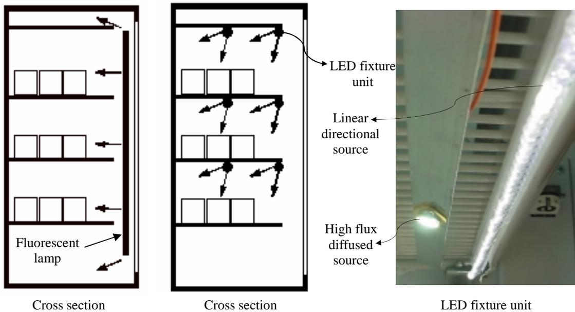
**Figure 4:** Schematic showing the light distribution with fluorescent lighting on the left and LED lighting on the right.
