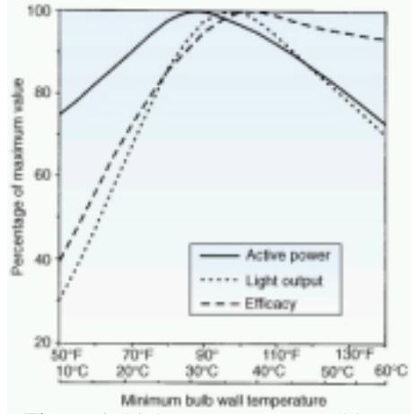
**Figure 1:** Light output versus ambient temperature curve for a typical fluorescent system <sup>[4]</sup>.
