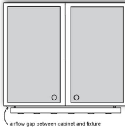
Creating an airflow gap between the cabinet and the fixture will help heat to escape, extending the life of the fixture.
