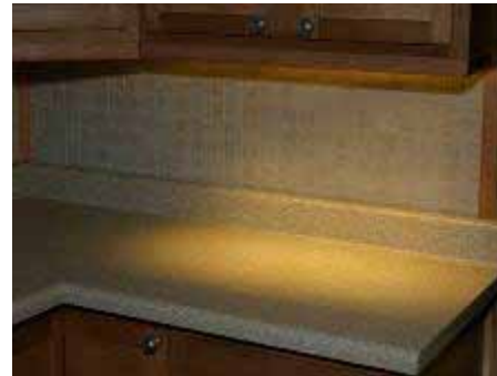
24 in. 5 mm LED “warm white” fixture Average illuminance: 153 lux Minimum illuminance: 7 lux Meets recommendation for critical tasks?: No Uniformity on counter: 22:1
