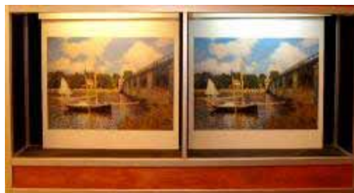
Warm CCT of 3000 K (left) and cool CCT of 6500 K (right).
