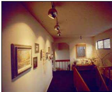
The accent light fixtures are aimed so that the scallops are uniformly aligned along the wall.
