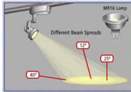
Examples of beam angles or beam spreads available for an MR16 lamp.
