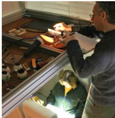
LRC researchers test halogen and LED reading lights in a mock aircraft cabin in a laboratory.
