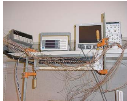
Figure 3: Thermocouples connected to jack panel and Agilent channel multiplexer
